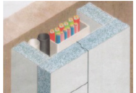
Pipe/Fire well/ Equipment partition
