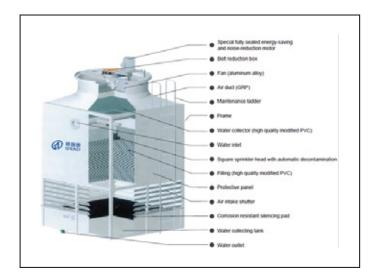
Square counter-flow stainless steel cooling towers are optimized in design of their structure and process on the basis of the traditional square GRP cooling tower
